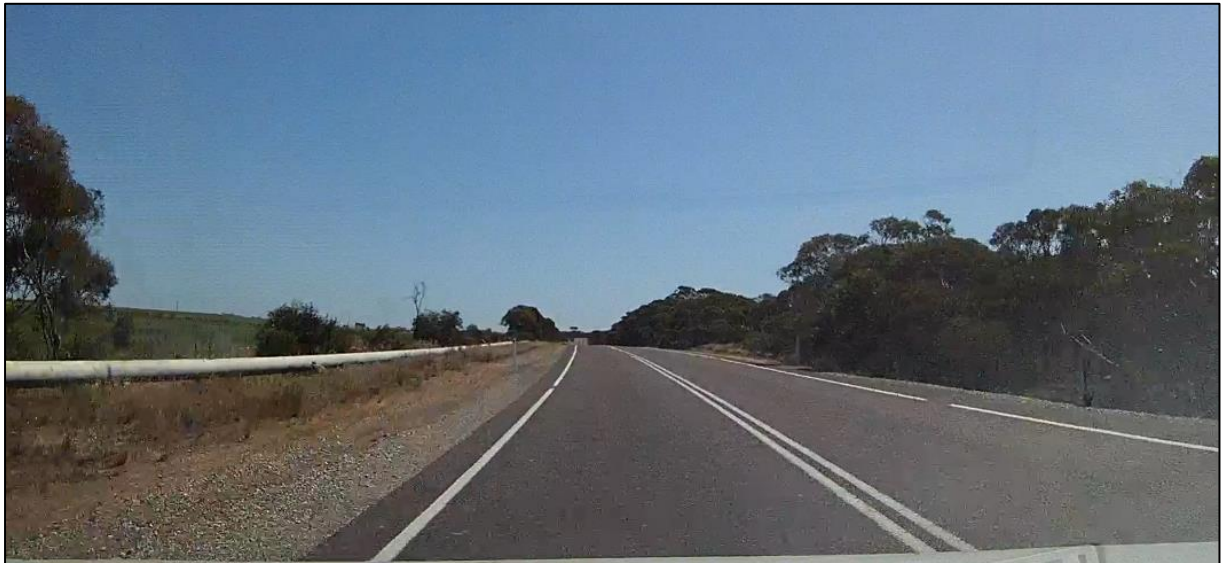
Figure 13 – Roadside hazards – High pressure pipeline (left) and edge drops with vegetation (right)
