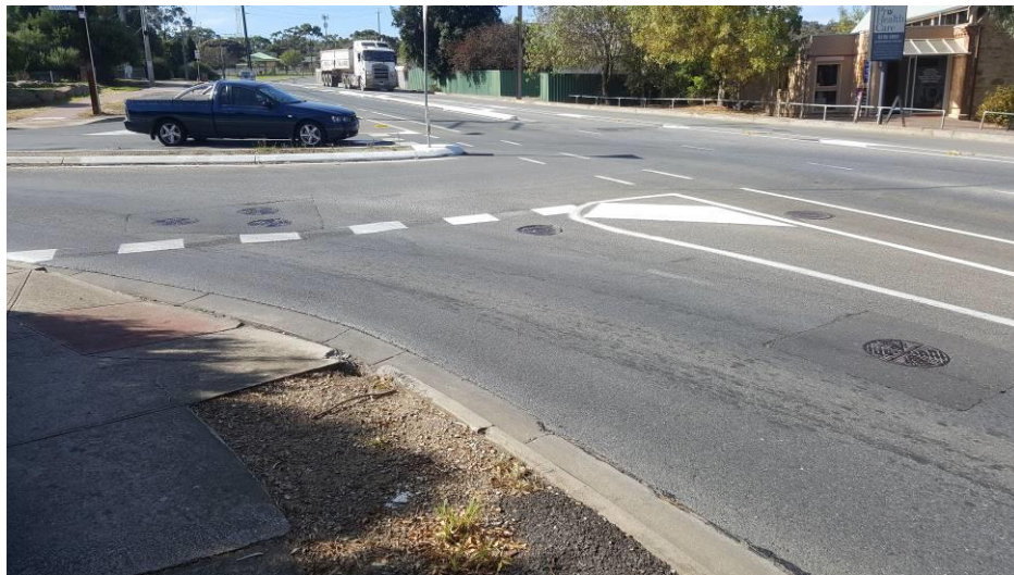
Figure 44: A holding line used at a slip lane in Hope Valley improved compliance with the give way rule without a sign
