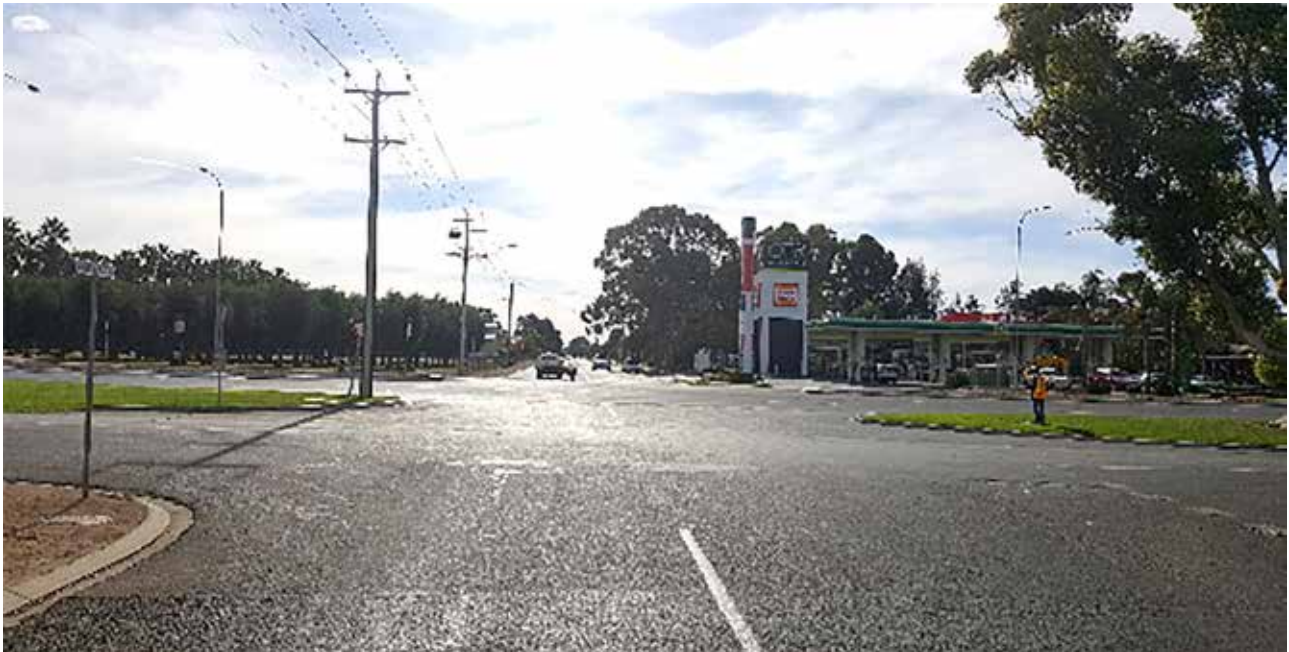
The north bound give way sign is particularly concealed by the stable pole and the upcoming give way condition is unclear
