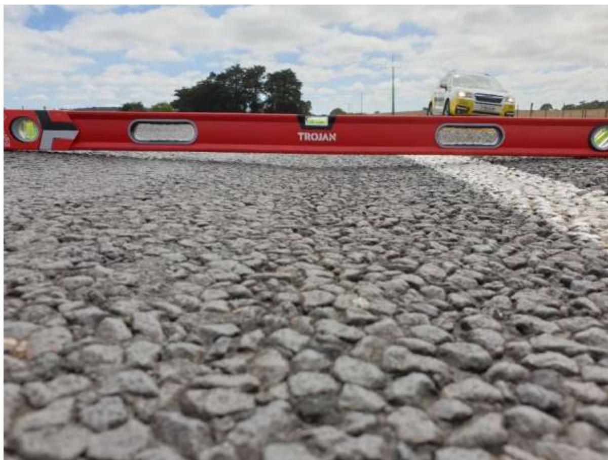
Rut depths measured on Glenelg River Road at Ob Flat
