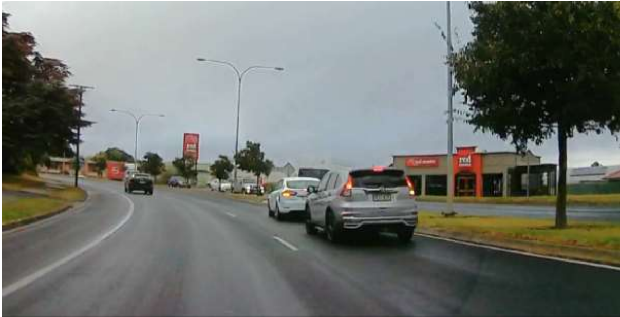
Vehicle queueing to make a U-turn frequently block the right lane of Jubilee Highway
