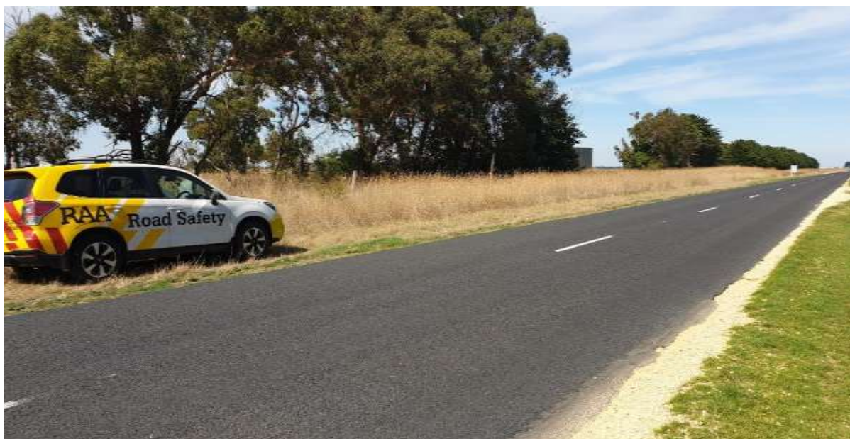
Narrow lanes and lack of shoulder seal south of Clay Wells
