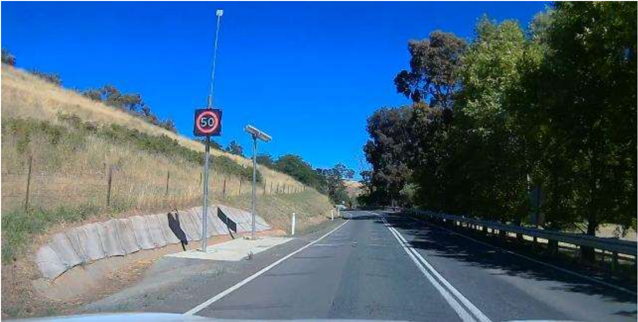
Figure 84: The RJAWS reduces the speed limit on Cudlee Creek Road when a vehicle is entering from the side road
