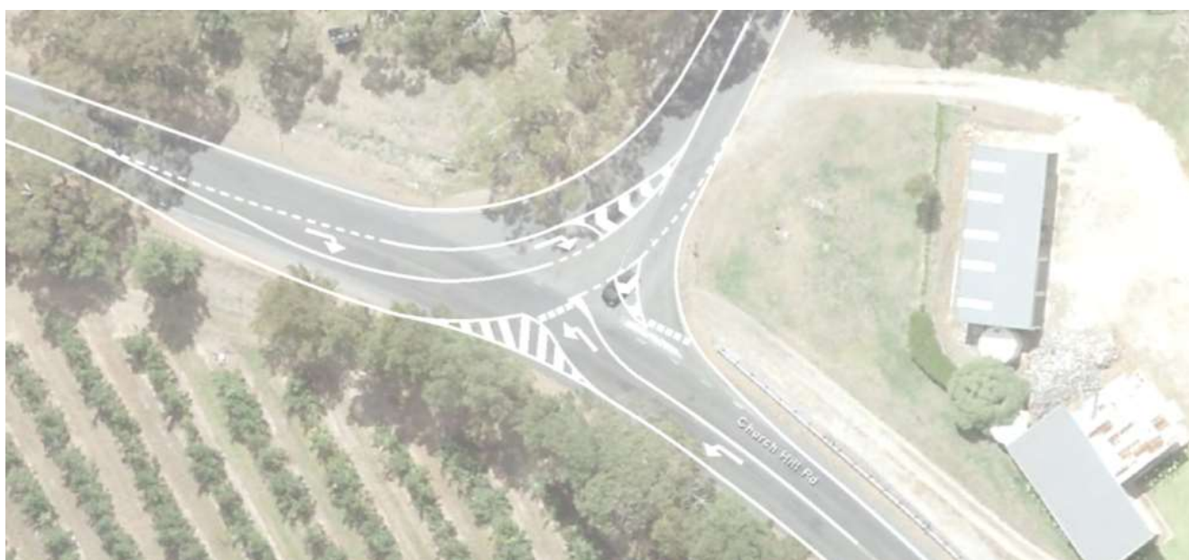
Figure 91: 'Modified T' intersection concept for the intersection of Church Hill Road and Old Mount Barker Road
