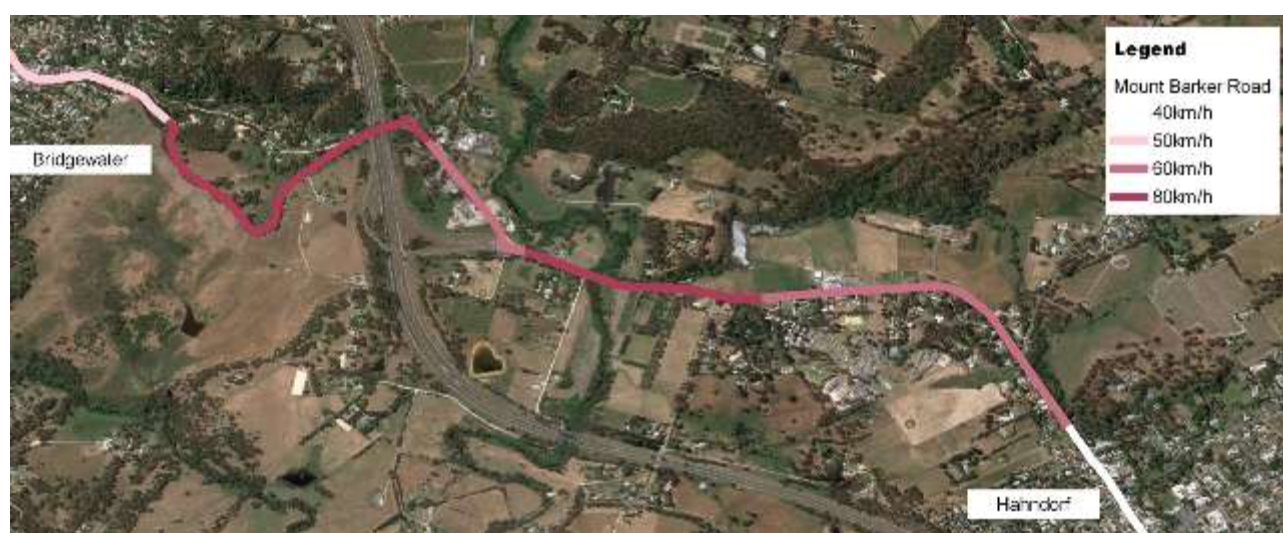
Figure 54: Variation in speed limits on Mount Barker Road between Bridgewater and Hahndorf
