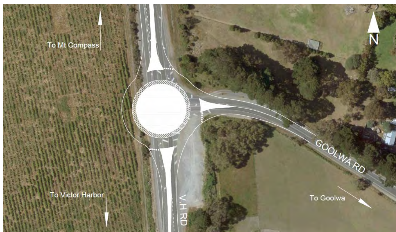
Figure 58: RAA concept sketch of a roundabout at the Victor Harbor Road/Goolwa Road intersection (22m central island radius used)
