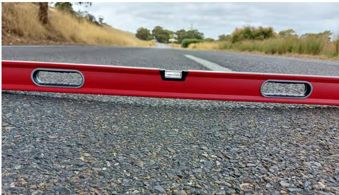
Figure 82: Rut depth on Pages Flat Road
