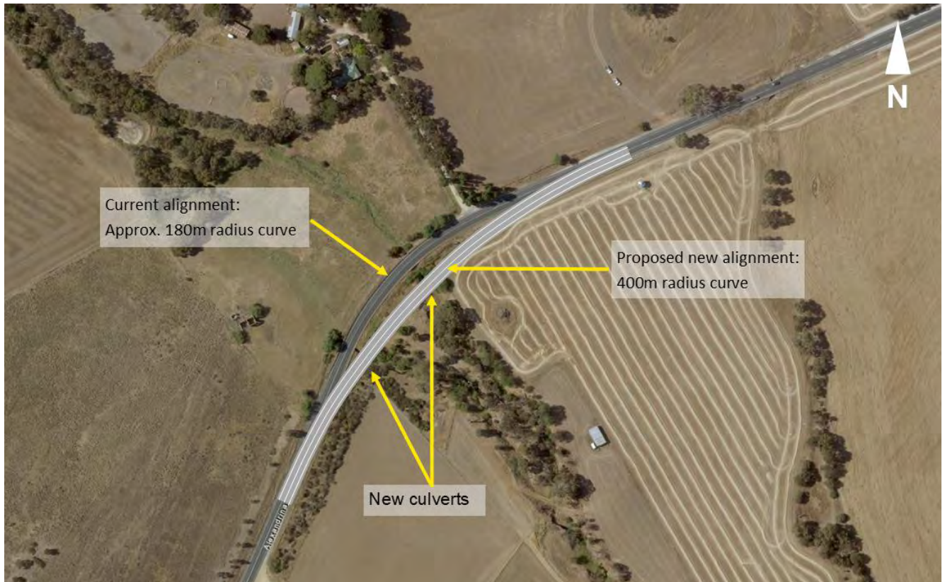
Figure 48: RAA proposed curve realignment to improve safety at the Jackson Creek Bridge
