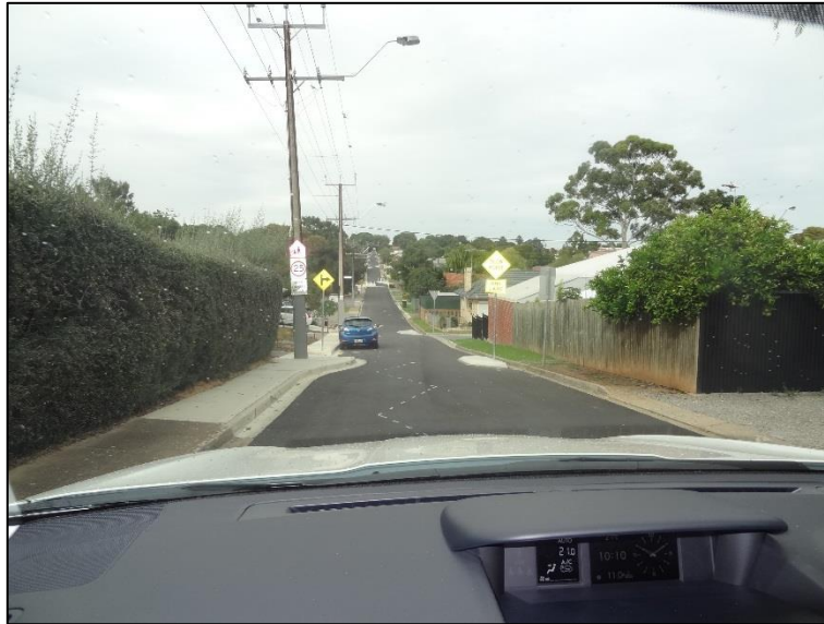
Figure 8 – The change of priorities are counter intuitive to the road user. The number of “Slow Point” warning signs may result in the “Road continues left/right” warning signs being disregarded. Priority signage (Give Way & warning signs) should perhaps be more prominent.
