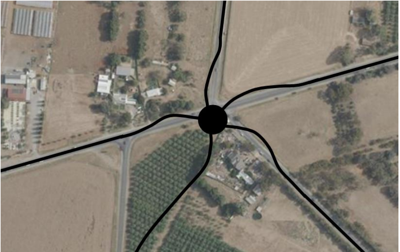
Figure 90: Layout sketch of a single roundabout treatment resulting in more significant land acquisition impacts.
